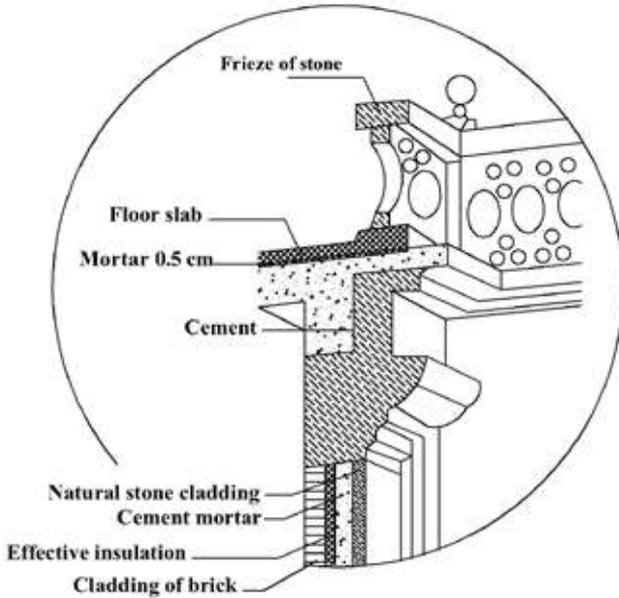
Il. 6. Section through the wall, showing the layers of building materials in French Mandate period (scheme credit H. Abass)
