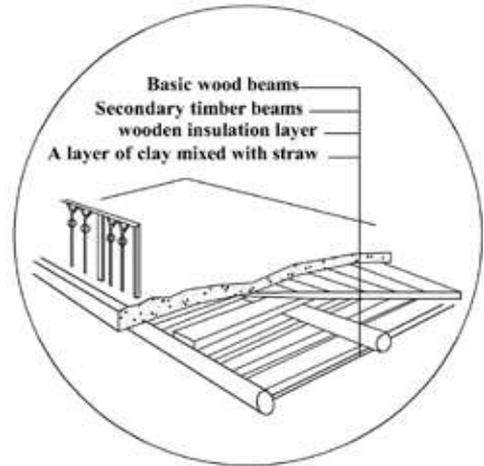
Il. 5. Traditional constructive isometric section (scheme credit H. Abass)
